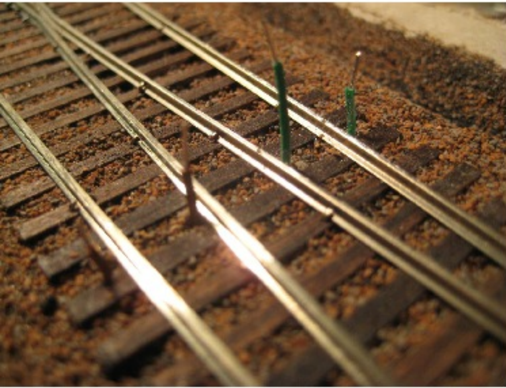
Closure rail wiring
